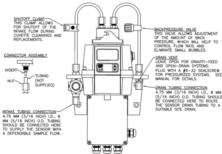
Figure 4: Recommended Plumbing for the Instrument
