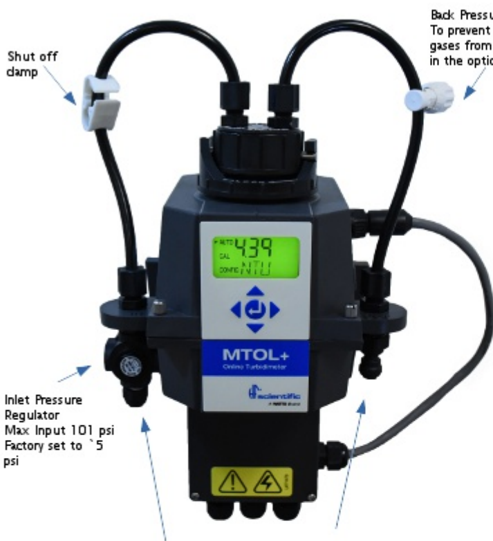
Sample Inlet and Outlet 1/4" OD push to connect fittings
