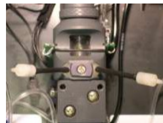
Remember to install the new pump tubes and check valves before re-assembling the reagent pump.
